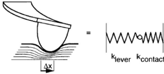
Figure 8. Lateral stiffness in FFM. The contribution of the tip is neglected (from [45]).
